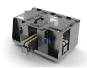
Bottles and cans are transported lying down and can be redirected and separated into three fractions on a minimal footprint. The number of fractions can be increased by cascading several sorting stations. The sorting station is therefore the direct interface between the reverse vending machine and the collecting/compacting point.
